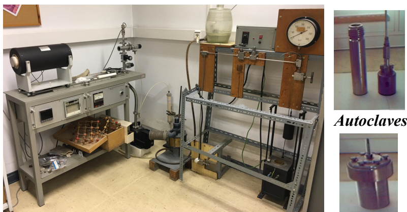
Figure 3: Left: vacuum or gas furnace (CNRS). Right: Hydrothermal synthesis system. (M.Á. Alario Franco & Emilio Morán)
