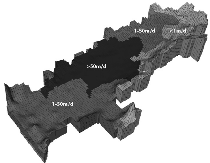
Fig. 5. The numerical model caters for geological and hydrogeological heterogeneities. This figure represents the distribution of time-independent hydrogeological parameters for the topmost model layer (horizontal hydraulic conductivity).
