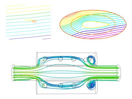
Figure 1: Stream function around a two-pieces airfoil, namely solution of a Dirichlet problem by the Chimera method converged in 4 iterations. Below, solution by freefem3d of the Navier-Stokes equations in 3D in a metro station when the train enter.
